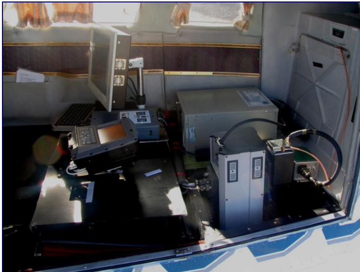
Figure 1. AISA-Eagle Hyperspectral and FLIR SC640 system used for aerial flight campaign.
