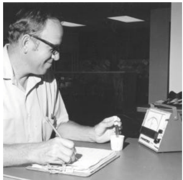
Loyal Quandt is using a pH meter to determine the soil pH. Lancaster County, 1973.
