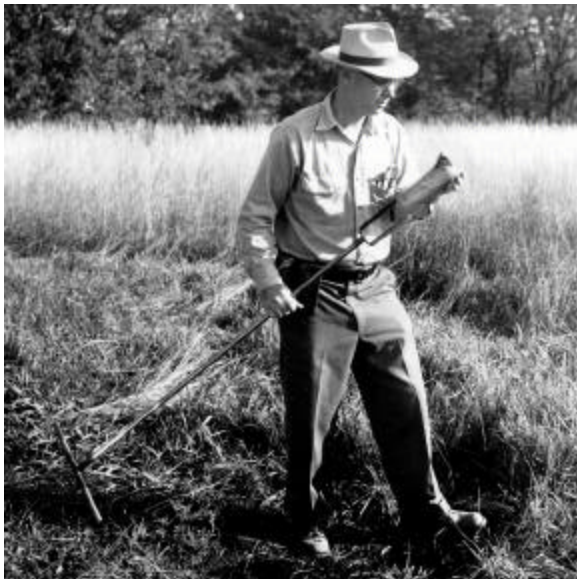
Loren Greiner using bucket type auger to examine soils. Pawnee County, 1957.
