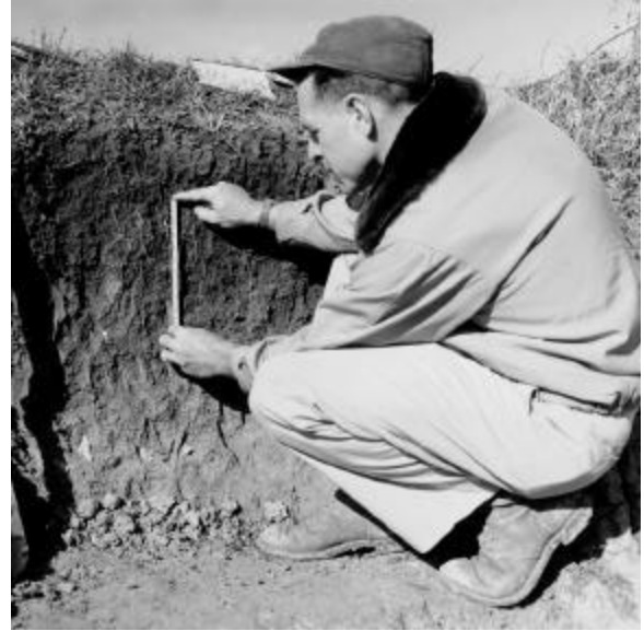
A soil scientist measures thickness of soil horizons to record in the soil description. 1959.
