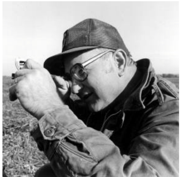
Dean DaMoude using Abney hand level to determine slope of land.
