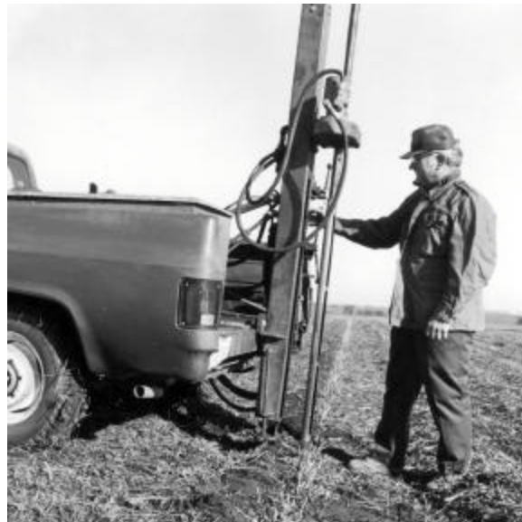
Dean using Giddings probe mounted on pickup to examine soils.
