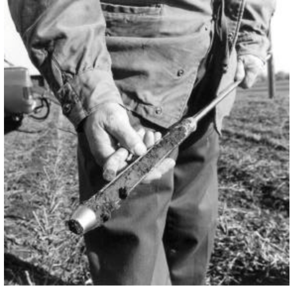
Dean is showing a close up of the soil core taken with the hand probe.
