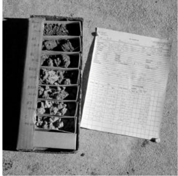
Example of soil correlation tray used to collect soil samples for soil correlation as part of the soil survey process.
