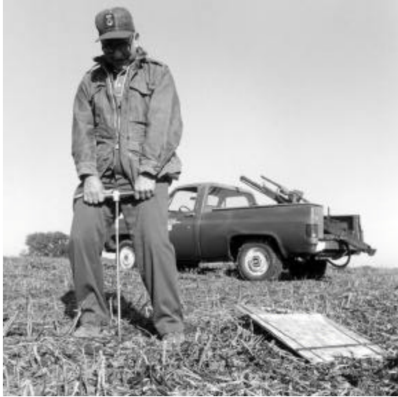
Dean DaMoude using hand probe to take a core of surface soil as part of field work for Saline County, 1981.
