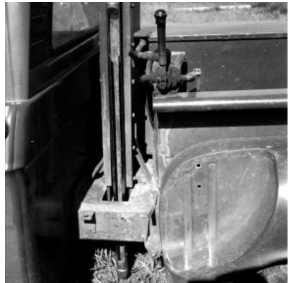
Close up of power probe used extensively by soil scientists in accelerating soil survey mapping.
