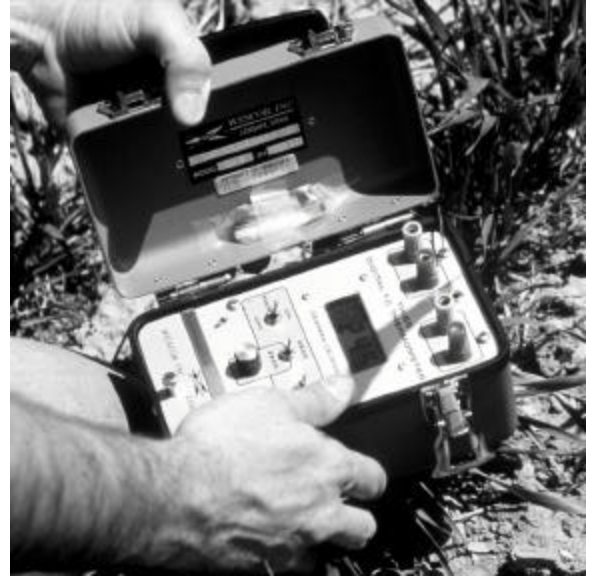
Soil scientists measuring soil temperature with a Thermocouples. Cheyenne County, 1984.
