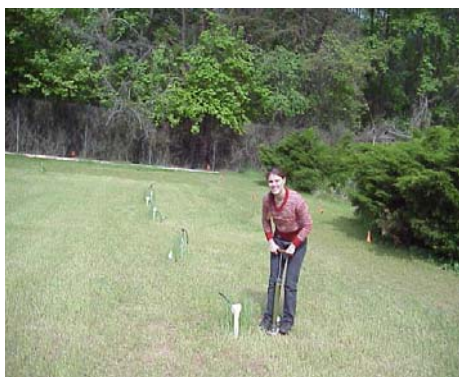
Student Intern taking water samples from lysimeters
