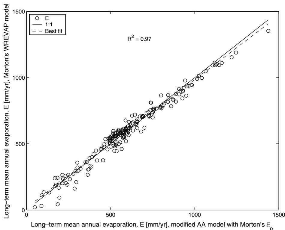
**Figure 7** Regression plot of the modified AA and WREVP model estimates of long-term mean annual evaporation for the 210 SAMSON stations. The modified AA model, with the  $\gamma/\delta(T_e)$  term, now employs the Morton  $E_p$  estimates.
