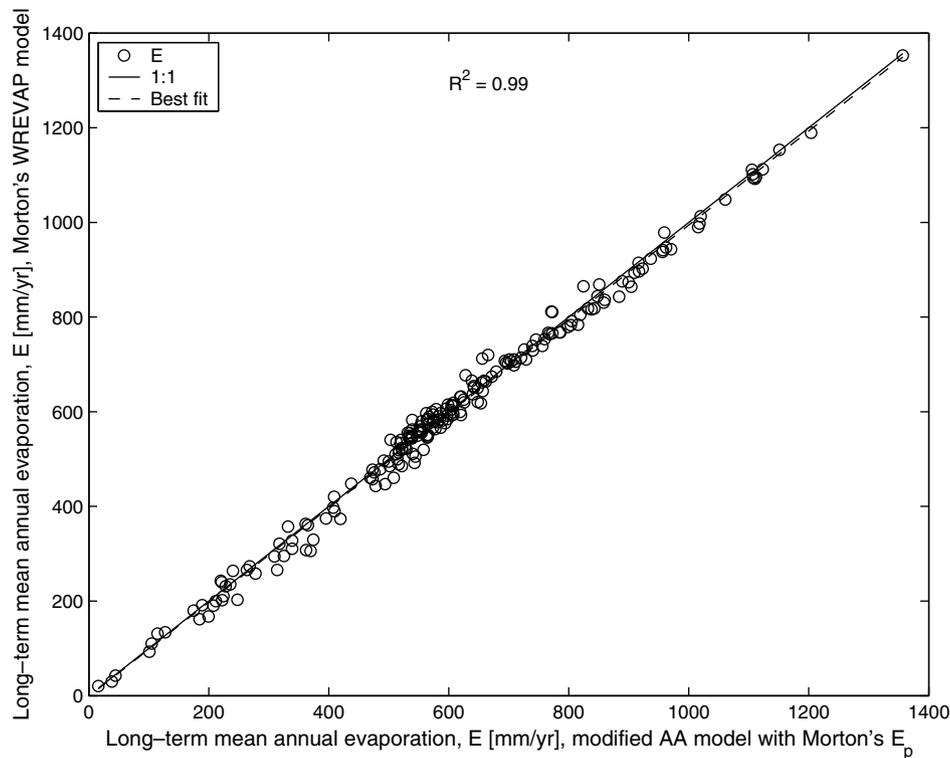
**Figure 8** Regression plot of the modified AA and WREVAP model estimates of long-term mean annual evaporation for the 210 SAMSON stations. The modified AA model now contains a constant (0.55) for the  $\gamma/\delta$  term and employs the Morton  $E_p$  estimates.
