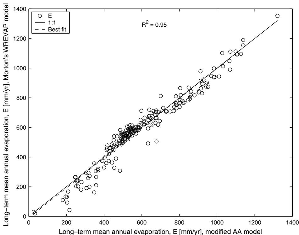
**Figure 11** Regression plot of the modified AA and WREVP model estimates of long-term mean annual evaporation for the 210 SAMSON stations. In the modified AA model now the  $\gamma/\delta$  term is replaced by a constant (0.55) and the wind function is the same as in Fig. 9.
