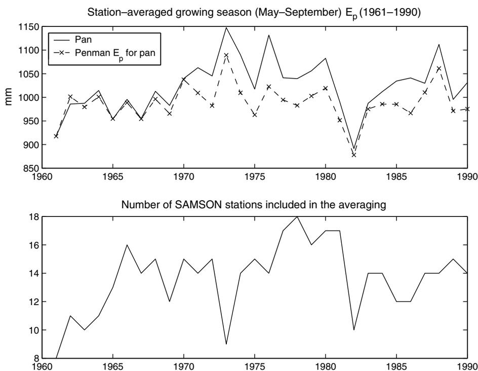
**Figure 12** Station-averaged growing-season class-A pan measurements and potential evaporation estimates of the Penman equation by year. The wind function in the Penman equation is the same as in Fig. 9. The number of stations fluctuates due to availability of data.
