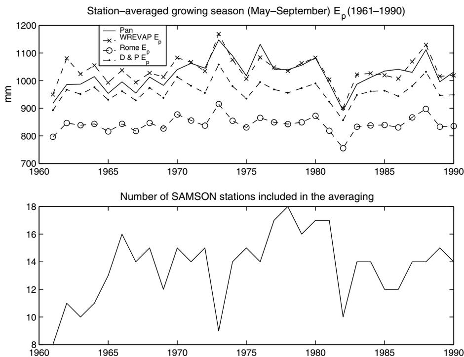
**Figure 5** Station-averaged growing-season class-A pan measurements as well as different potential evaporation estimates by year. 'Rome' and 'D & P'  $E_p$  denote the Penman-equation  $E_p$  by the Rome and the Doorenbos–Pruitt wind functions, respectively. The number of stations fluctuates due to availability of data.
