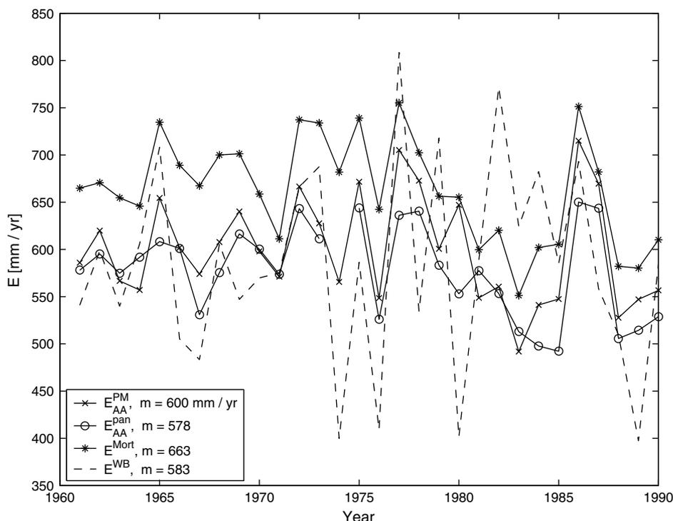
**Figure 15** Annual evaporation estimates for the Elkhorn watershed in Nebraska.  $E_{AA}^{pan}$ : evaporation estimate by the modified AA model with pan data;  $E_{AA}^{PM}$ : evaporation estimate by the modified AA model with the Penman equation values;  $E^{Mort}$ : evaporation estimate of Morton's WREVP model;  $E^{WB}$ : water-balance-derived evaporation;  $m$ : 30-yr mean value.
