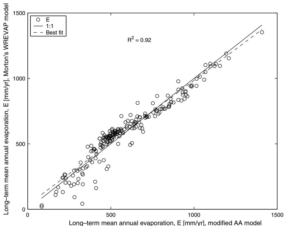
**Figure 10** Regression plot of the modified AA and WREVAP model estimates of long-term mean annual evaporation for the 210 SAMSON stations. The modified AA model employs the Penman  $E_p$  values with the same wind function as in Fig. 9.
