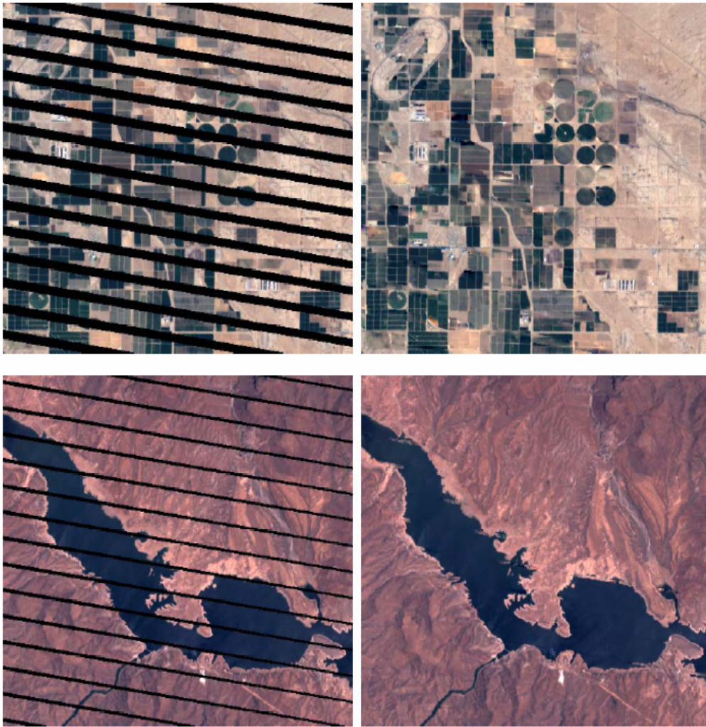
Figure 6. Examples of SLC-Off and SLC corrected Landsat 7 ETM+ scenes using bands 3, 2, 1. SLC-Off scene is path 36 row 37, acquired 6/24/2003. SLC corrected scene is the same image, filled with matched data acquired 7/7/2002. (Scaramuzza et al. , 2004)
