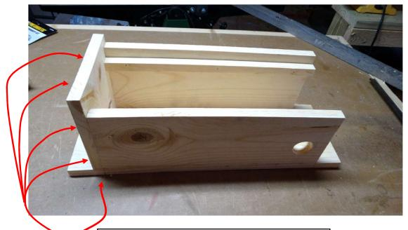
Two screws/nails each attaching it to each side. One screw/nail attaching it to the back board (proximately in the middle).
