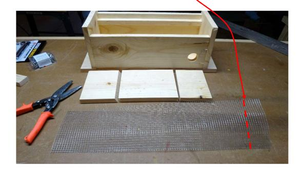
For the next cut, the bottom screen portion should be approximately  $\frac{1}{2}$ " above bevel. After cutting the hardware cloth, turn it  $180^{\circ}$  so that the relative smooth edge will now be at the top.
