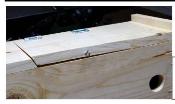
Drill a pilot hole and attach the "eyelet" portion of the hookand-eyelet.
