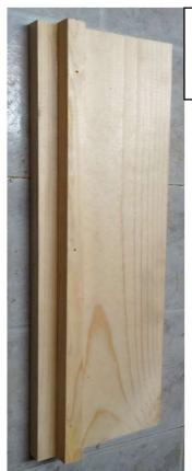
The front panels will rest on this added strip of wood—with the hinges on this side of the box.
