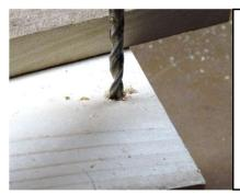
After drilling those holes, remove the bat board and drill through the back board holes you just created using a larger drill bit (5/8 to 3/4" inch). This "slop" you are creating will make it much easier to hang the box...and remove it if you need to make repairs or clean it out periodically.
