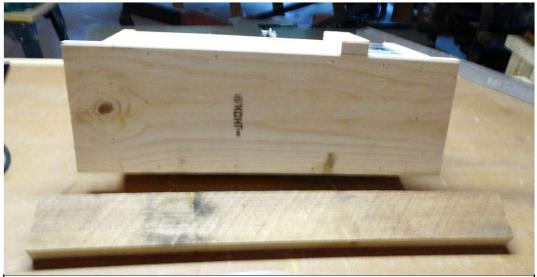
Use a thicker board as the "bat" board. Can be treated or untreated. It will eventually be nailed to the tree. It should extend  $1 \frac{1}{2}$ -2" beyond each end of the back board. Width should be  $2 \frac{1}{2}$ -3".
