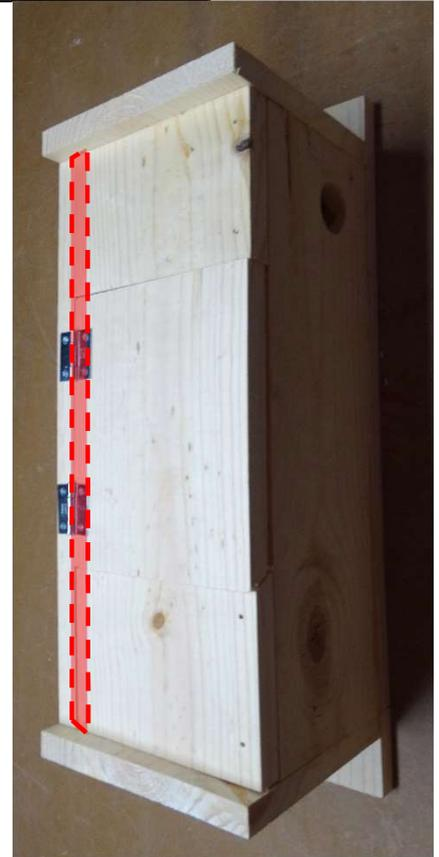
**Suggest you assembly right side (with the hole) to the back panel first. Glue and nail.**
