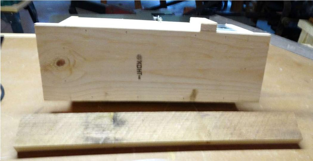
Use a thicker board as the “bat” board. Can be treated or untreated. It will eventually be nailed to the tree. It should extend 1 ½-2” beyond each end of the back board. Width should be 2 ½-3”.
