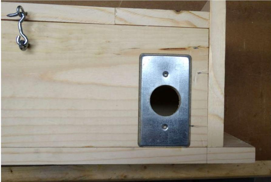
Be sure to use short enough screws so that they do not penetrate all the way through the wood. Ok to screw down until metal plates bows in a bit.
