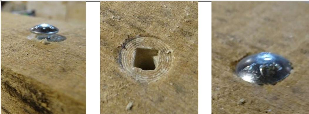
This set of images shows the carriage bolt through the “bat” board and the “back” board with a washer and nut. Once on the tree, you will tighten the nut down (hand-tightening is sufficient) as shown on the right.
