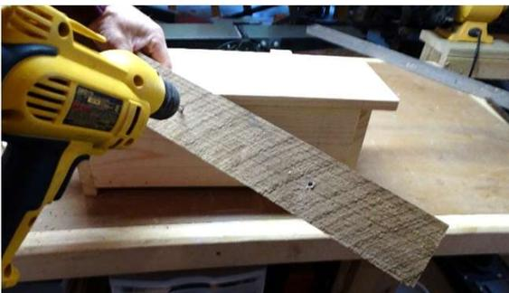
Drill 2-3 holes in the bat board that are a) large enough for the spike-size nail to easily go through (this will eliminate splitting this board when it comes time to attach it to the tree) and b) approximately 1” from what will be the ends of the bat board. Check schematic again for this general positioning of these holes.
