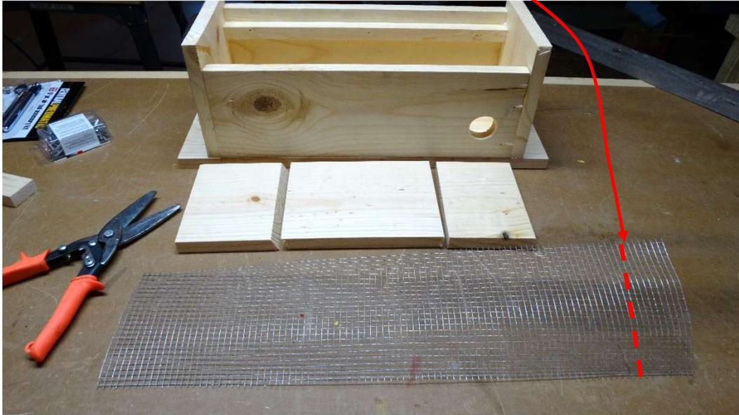
For the next cut, the bottom screen portion should be approximately  $\frac{1}{2}$ " above bevel. After cutting the hardware cloth, turn it 180° so that the relative smooth edge will now be at the top.
