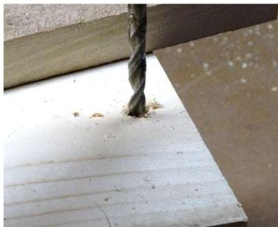
After drilling those holes, remove the bat board and drill through the back board holes you just created using a larger drill bit ( $\frac{5}{8}$  to  $\frac{3}{4}$ " inch). This “slop” you are creating will make it much easier to hang the box...and remove it if you need to make repairs or clean it out periodically.
