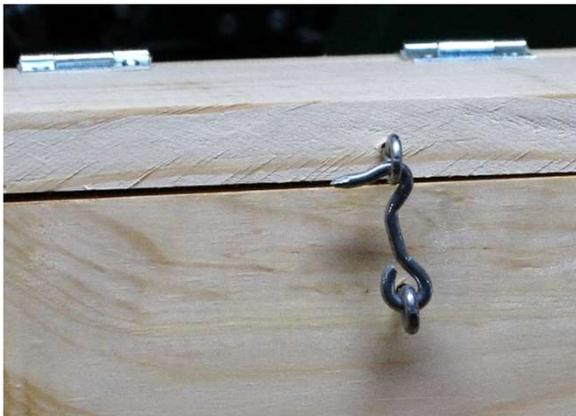
Drill a pilot hole and attach the “hook” portion of the hook-and-eyelet. Should have a “snug” fit.
