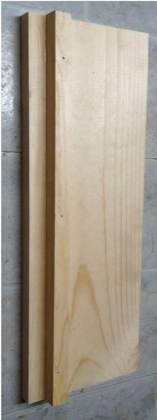
The front panels will rest on this added strip of wood—with the hinges on this side of the box.
