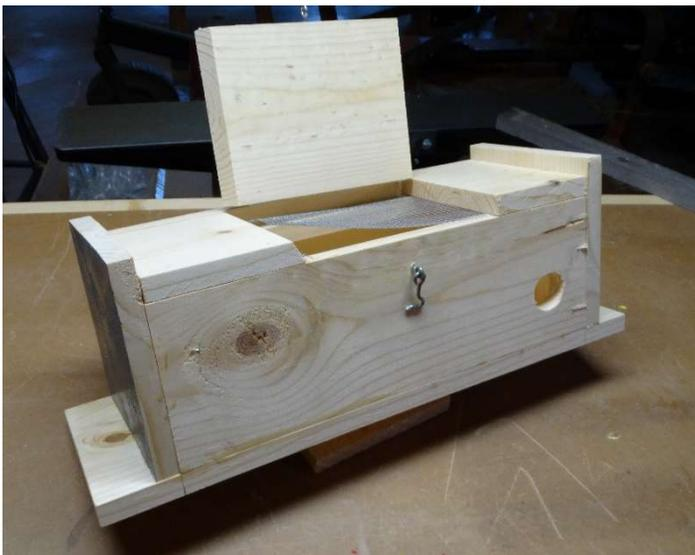
**Add the metal plate cover—centered over the hole. Add the cleat below the metal plate.**
