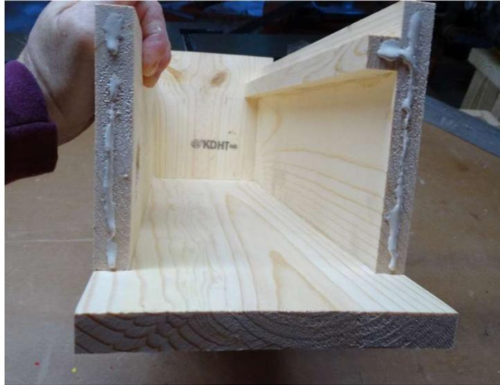
Same as attaching bottom: Two screws/nails each attaching it to each side. One screw/nail attaching it to the back board (proximately in the middle).
