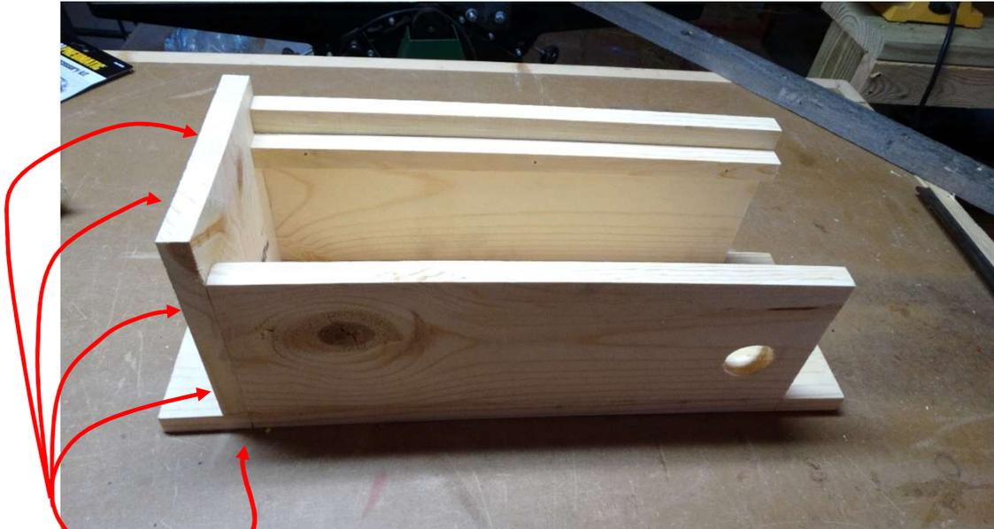
Two screws/nails each attaching it to each side. One screw/nail attaching it to the back board (proximately in the middle).
