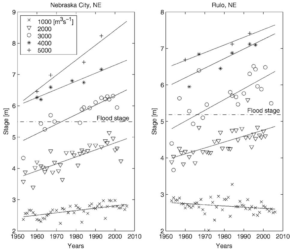
**Fig. 2.** Specific-stage diagrams of the Missouri River at Nebraska City and Rulo, Neb. with linear trend functions fitted. Note that data for each year are for hydrologic years that start October 1 the previous year and end September 30 the year shown.
