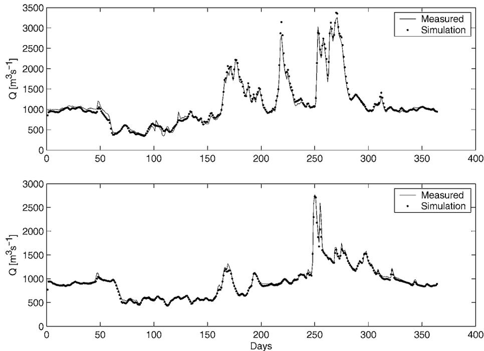
**Fig. 3.** Measured and simulated daily mean discharges of the Missouri River at Rulo, Neb.: (a) hydrologic year 1953; (b) hydrologic year 1995
